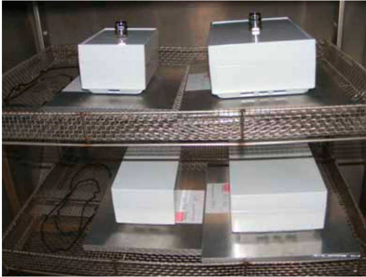
Figure 1 Loading by Rapid Changes of Temperature
