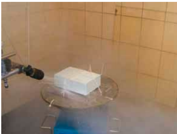
Figure 12 Exposition IP X9K, 30°, exemplarily
