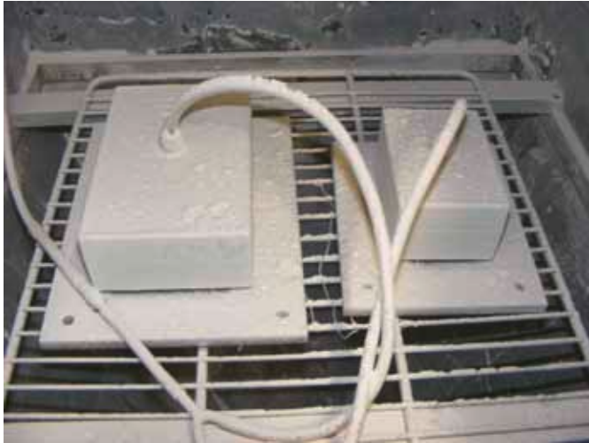
Figure 8 Loading by dust IP 6X
