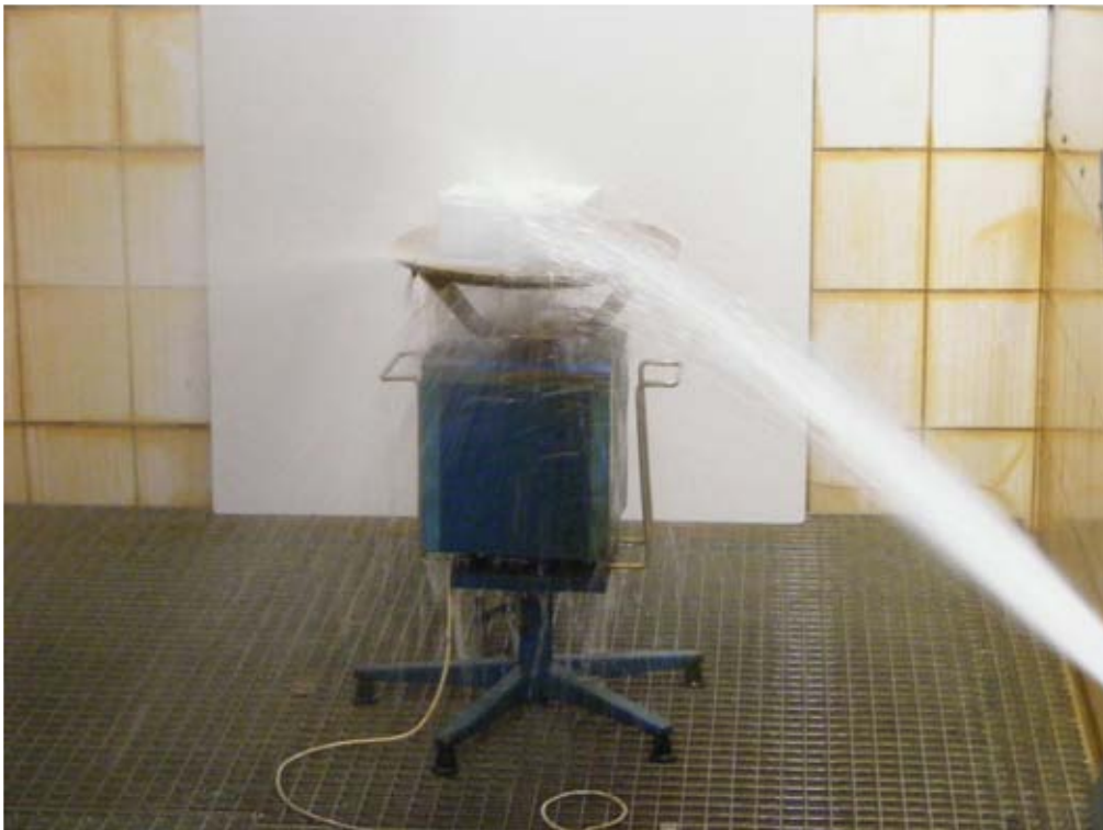
Figure 2 IP Code X6, loading by strong jet of water, exemplarily
